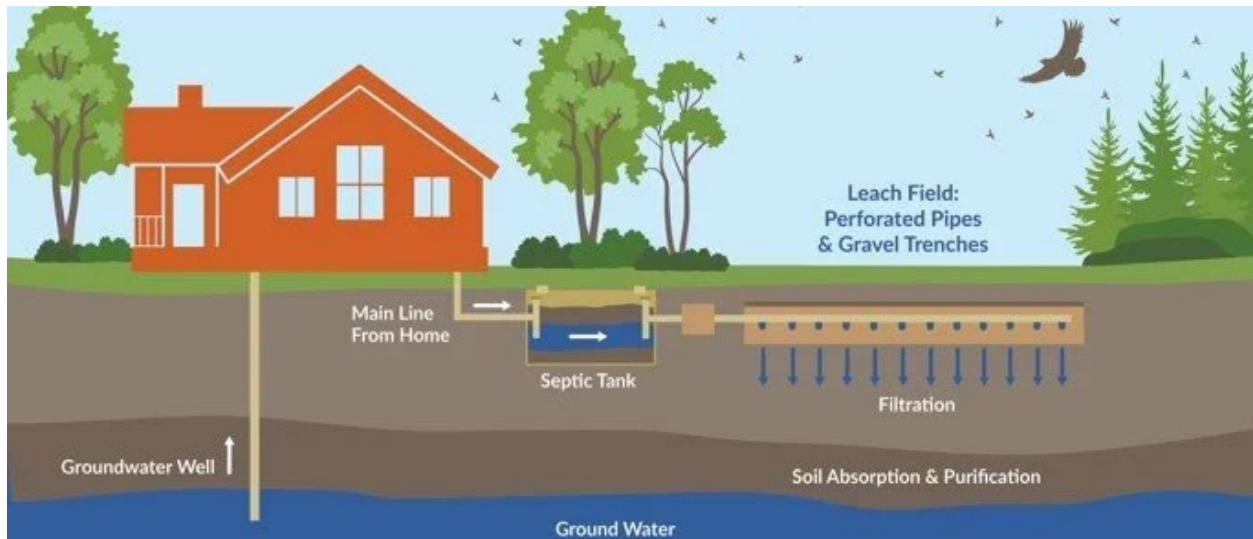
Figure 5. Illustration of a septic system and drain field. Source: https://www.lakesunapee.org/septic-systems .
